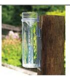
A RAIN GAUGE is an instrument used to gather and measure the amount of liquid precipitation over a set time.
